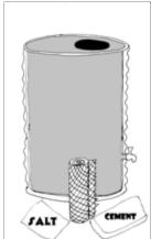
An old galvanised tank can be fixed by covering the inside with chicken wire. It can then be plastered with a mix of sand, cement and salt (to make it non-porous), and then left to dry.
