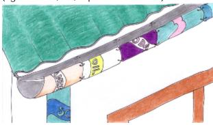
WARNING: Check that no paint is peeling off your roof which will contaminate your water. If your roof is made of asbestos or thatch then you should NOT use this water for drinking.
